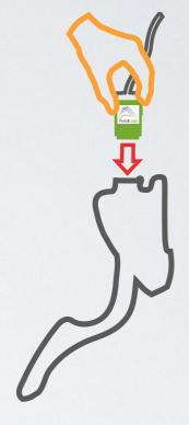
With ignition off, unsnap wire harness from accelerator pedal.
