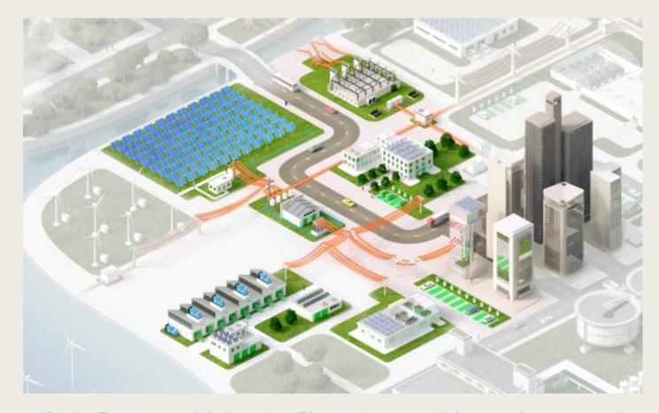
Duke Energy and Schneider Electric have collaborated on several microgrids. Above is a representation of what a microgrid would contain, including solar panels, battery storage, a power control unit, converters, and distribution lines
